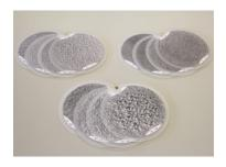
**article 990** (article 991+992) Degree of pilling, wovens and knits An objective evaluation of the pilling tendency of woven cloth and knitted fabric is a broad requirement of the textile industry.
